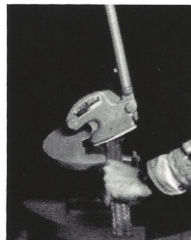
B-1 Beverly Shear; set to cut 1/4" flat braided ground cable ends and or to length.
