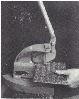
SS2 Shear; modified upper blade and frame; shown cutting nail plate stock to length or shapes for truss manufacture or other joining of wooden, etc. parts.
