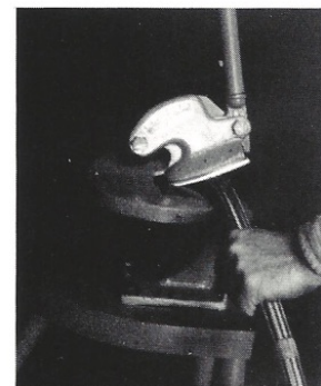
B-1 Beverly Shear; set to cut braided stock and/or braided covered hose to length and/or for end fittings.
