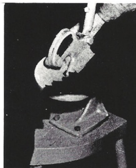
Beverly Shear Series; zig-zag cuts are easily made on a throatless shear because movement of the work is unhampered by a throat or center post.
