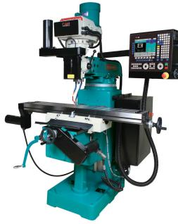
An affordable, heavy-duty CNC Vertical Mills with a wide range CNC control and the advantage of Electronic Variable Speed. Affordable standard heavy-duty Electronic Variable Speed (EVS) Milling Machines. Head mounted controls with LCD spindle speed display.
