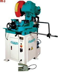
High-production Ferrous Cutting Semi-Automatic, Pneumatic Vise and Manual, burr-free cutting Cold.
