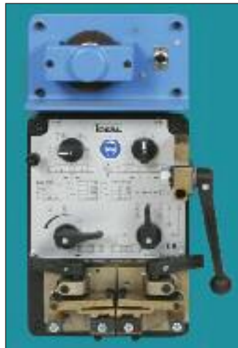
Clausing Installed Welder, Shear, Grinder (welders only go to 1")
